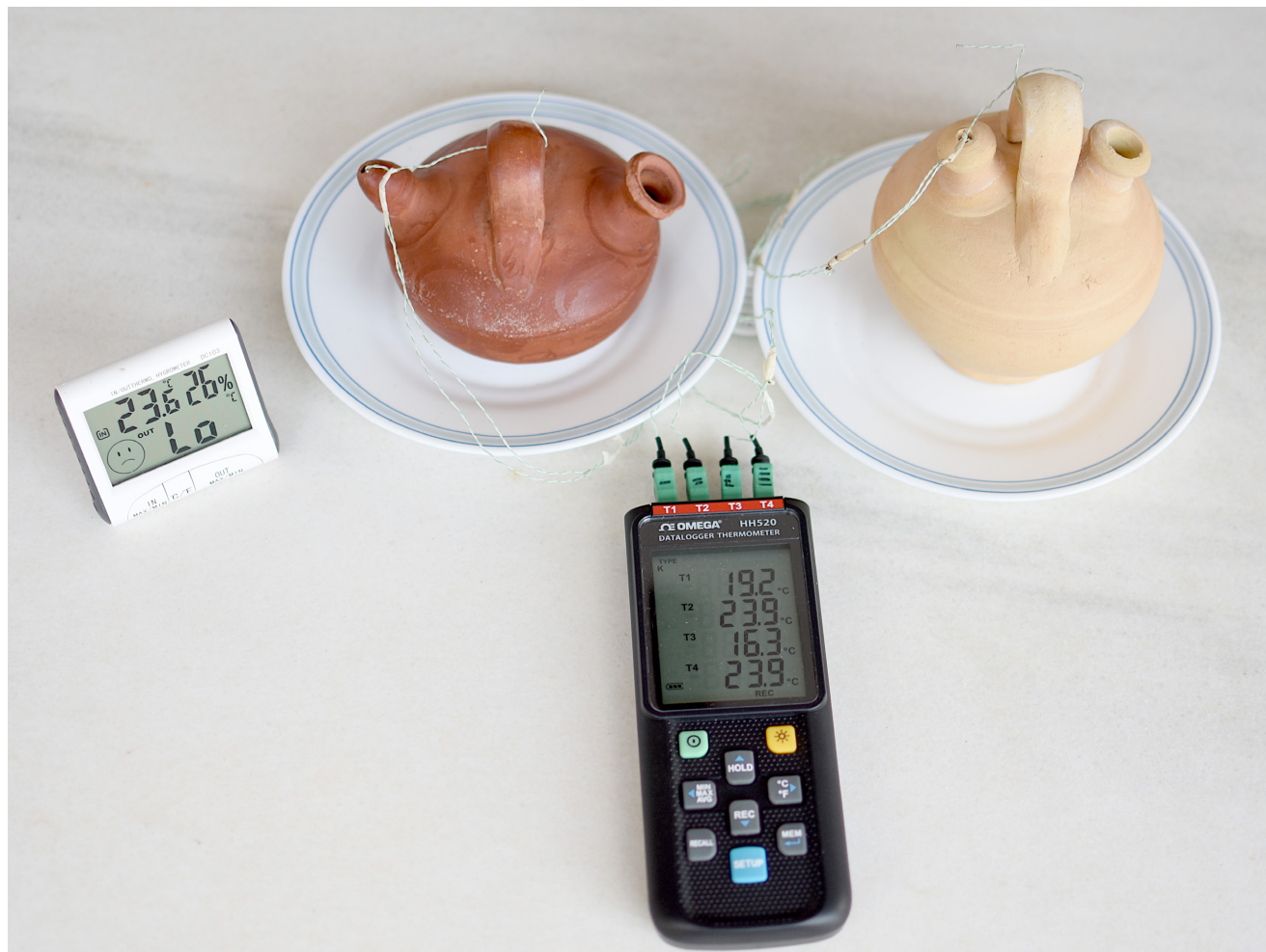
Photo 2. The large thermal deficit inside Carlina corymbosa flowerheads at high ambient temperatures was most likely achieved through a “botijo” effect. Sweating pitchers made of porous clay ( botijos in Spanish) as those shown in the picture have been used traditionally as a water-chilling technique by human cultures from the Mediterranean Basin and other hot-dry areas of the world. Through intense water evaporation, they can achieve temperature drops inside of up to 20°C relative to the ambient, depending on clay porosity and environmental conditions (temperature, humidity, wind speed). The display of the data logger in the picture shows the temperatures of the water inside the less-porous red (Channel T1, 19.2°C) and highly-porous yellow (Channel T3, 16.3°C) botijos, and the respective air temperatures outside (Channel T2 and T4, 23.9°C). Photo credit: Carlos M. Herrera.
